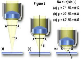
The next figure shows the difference in depth of field between a low and high power objectives.
